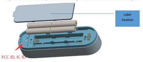
Step 2: Close the back cover of the product. Battery cover and back cover were fixed by snap, Difficult to open by hand, need to use tools to pry it open
