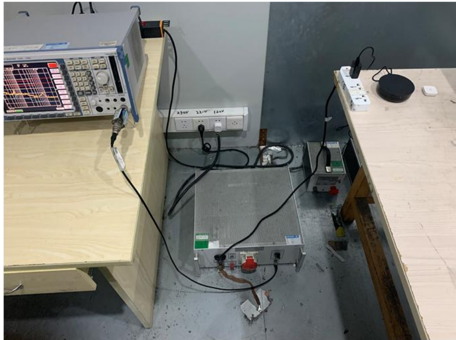
Conducted Emission Test Setup
