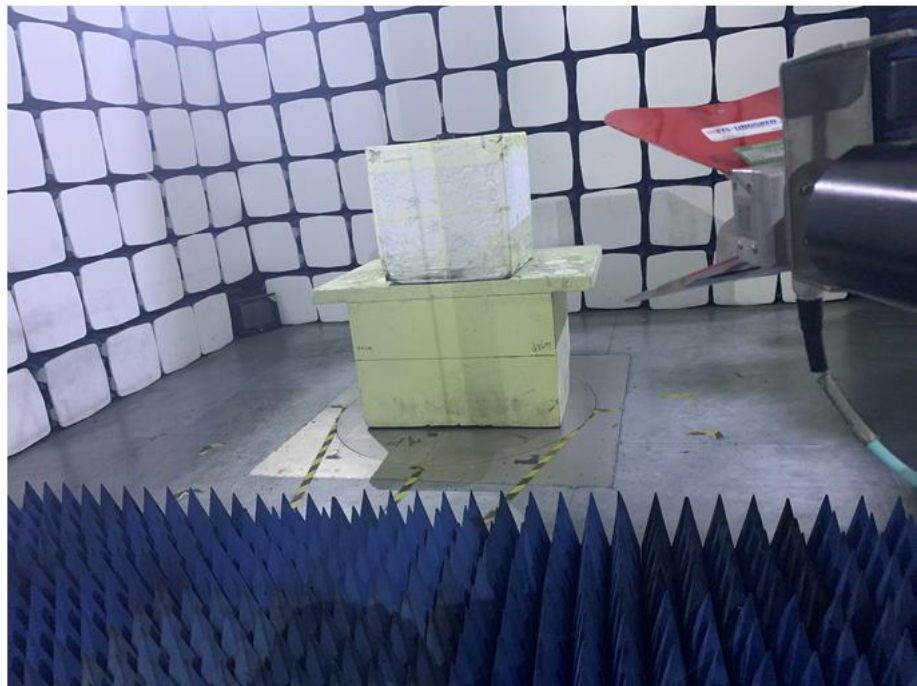
Radiation Emission Test Setup (1GHz to 18GHz)
