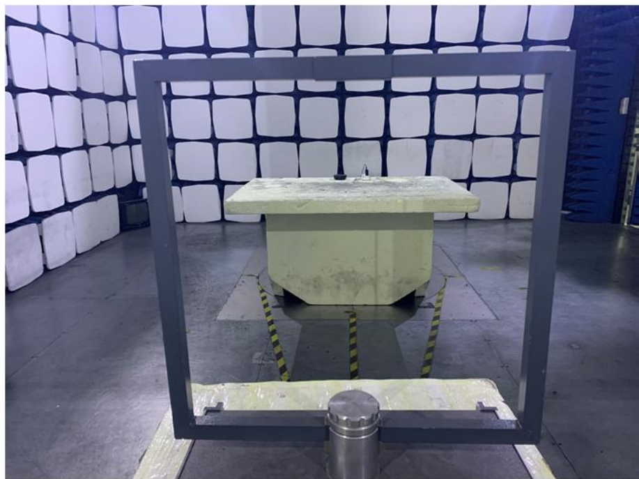
Radiation Emission Test Setup (Below 30MHz)
