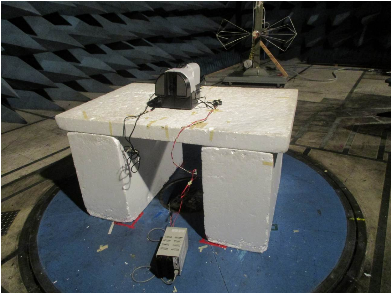
Figure 3: Radiated Emissions – Back View – 30 MHz – 200 MHz
