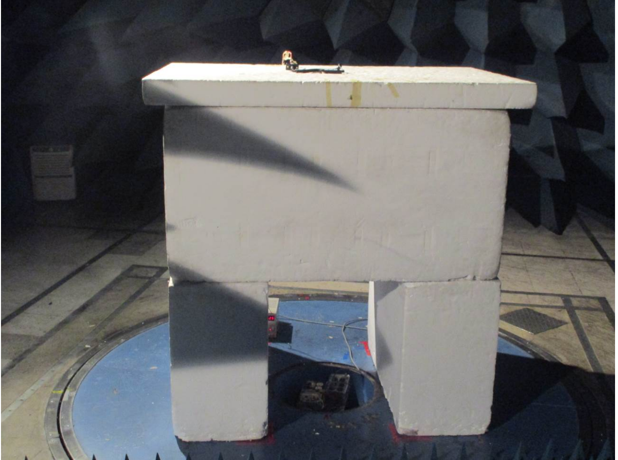
Figure 5: Radiated Emissions – Front View – Above 1 GHz – Flat
