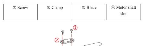
The process of propeller disassembly is as follows. First, remove the screws. Then rotate the clamp of the Type A propeller rightwards or the clamp of Type B propeller leftwards 45 degrees, then remove the clamp. Finally, remove the propeller.
