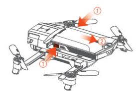
Align the battery with the locking slot of the body, and insert the battery by pushing forwards.
