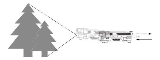
The accuracy of the vision position system is likely to be influenced by light intensity and surface of obstacles, and ultrasonic positioning may be inaccurate if the drone flies close to sound-absorbing materials. Therefore, be careful not to rely on the vision position system in the following conditions:
