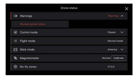
3. Start magnetometer calibration. Hold the aircraft and rotate it clock-wisely and horizontally. Observe the color of the LED indicator light in the aircraft and go to the next step when the LED indicator turns solid white light. Otherwise, please return to the step 2.
