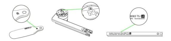
The process of propeller installation is as follows. First, select the same type of propeller as per the letter on the motor. With the letter facing upwards, press the blade into the clamp. Then press the clamp into the slot of the motor shaft, and turn the Type A propeller leftwards 45 degrees and the Type B propeller rightwards 45 degrees, until the holes at the two ends are aligned with the stop pins.
