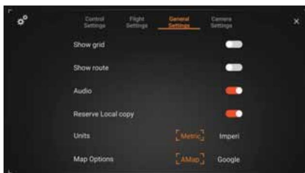
In this page, settings can be adjusted for units of the parameters, whether to show the grid, whether to show the flight track and whether to broadcast the sound effect. This is also where you can format the microSD card for the camera.
