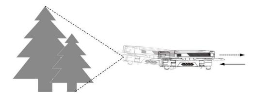
The accuracy of the vision position system is likely to be influenced by light intensity and surface of obstacles, and ultrasonic positioning may be inaccurate if the drone flies close to sound-absorbing materials. Therefore, be careful not to rely on the vision position system in the following conditions:
