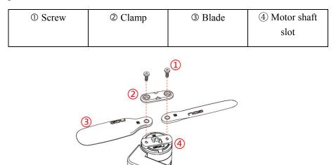
The process of propeller disassembly is as follows. First, remove the screws. Then rotate the clamp of the Type A propeller rightwards or the clamp of Type B propeller leftwards 45 degrees, then remove the clamp. Finally, remove the propeller.
