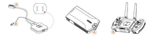
Input voltage: 100-240V Charging time: less than 2.5 hours (A+B)
