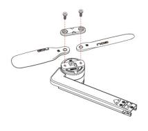
2 small set screws and a second proprietary locking mechanism, the props on the  $O_2$  will ensure they stay secured during flight.
