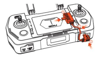
2. Adjust the length of remote controller, clamp the mobile phone into the appropriate position, and connect the other end to the mobile phone's charging interface.
