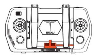
The remote comes equipped with a Lightning cable by default. If requires, please replace it with the Micro USB cable.
