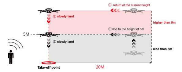
If the aircraft is over 20m away from the return point, the aircraft will rise to the preset height (if the current height is above the set height, the aircraft will fly at the current height), fly directly above the return point, and then slowly land.
