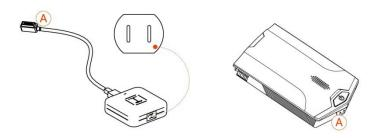
Input voltage: 100-240V Charging time: less than 2 hours
