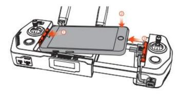
3. After flying, remove the mobile phone and fix the data cable back into the slot.
