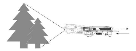
The accuracy of the vision position system is likely to be influenced by light intensity and surface <u>of obstacles</u>, and ultrasonic positioning may be <u>inaccurate if</u> the drone flies close to sound-absorbing materials. Therefore, be careful <u>not to rely on</u> the vision position system in the following conditions:
