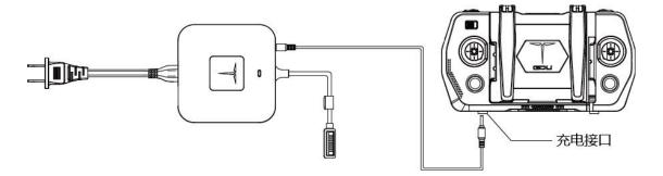
Only charge the remote controller in its OFF state. Check whether the remote controller is fully charged according to the charger's indicator light color. If the power indicator flashes in red, it means that the remote controller is being charged. If the power indicator shows a steady ON in green, it means that the remote controller has been fully charged. The charging duration is generally within 2 hours. A fully charged remote controller can be used for about 1.5 hours.
