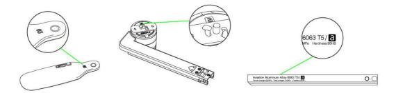
The process of propeller installation is as follows. First, select the same type of propeller as per the letter on the motor. With the letter <u>facing</u> upwards, press the blade into the clamp. Then press the clamp into the slot of the motor shaft, and turn the Type <u>A</u> propeller leftwards 45 degrees and <u>the</u> Type <u>B</u> propeller rightwards 45 degrees, until the holes at <u>the</u> two ends are aligned with the stop pins. Finally, tighten the screws.
