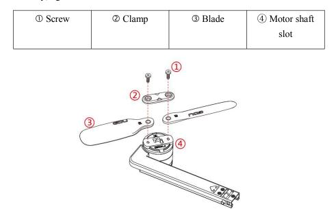
The process of propeller disassembly is as follows. First, remove the screws. Then rotate the clamp of <u>the</u> Type <u>A</u> propeller rightwards or the clamp of Type <u>B</u> propeller leftwards 45 degrees, <u>then</u> remove the clamp. Finally, remove the propeller.
