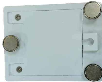
Figure 2 Magnets at Bottom of LAS-603
