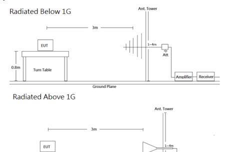
Radiated emission tests were performed in the 3 meters chamber test site, using the setup accordance with the ANSI C63.10-2013. The specification used was the FCC Part 15.209 and FCC 15.247 Limits.
