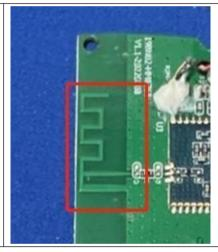
The antenna is PCB antenna. The best case gain of the antenna is 1.89 dBi.
