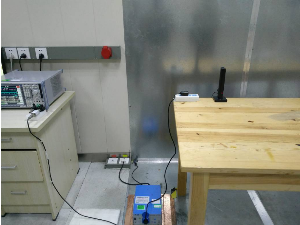
RADIATED EMISSION TEST SETUP BELOW 1G
