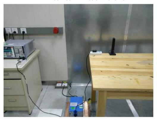
RADIATED EMISSION TEST SETUP BELOW 1G
