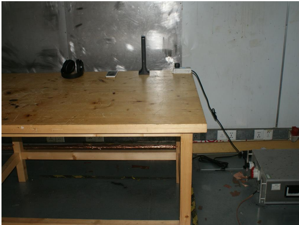
Photograph 6: Set-up for conducted emission test
