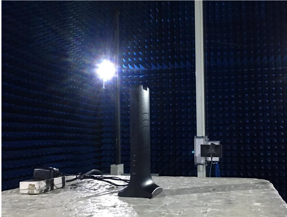
Photograph 3: Set-up for Spurious Emissions (1GHz-18GHz)
