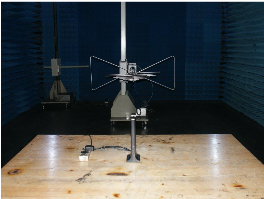
Photograph 2: Set-up for Spurious Emissions (30MHz-1GHz)
