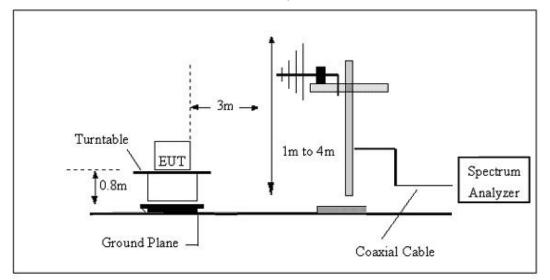
(C) Radiated Emission Test-Up Frequency Above 1GHz
