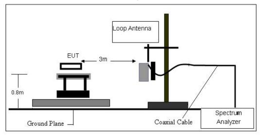
(B) Radiated Emission Test-Up Frequency 30MHz~1GHz
