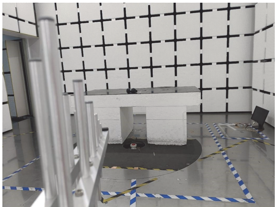
Radiation Emission Test Setup (30MHz to 1GHz)
