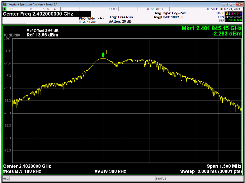
Tx. Spurious NVNT 1-DH1 2402MHz Ant1 Emission
