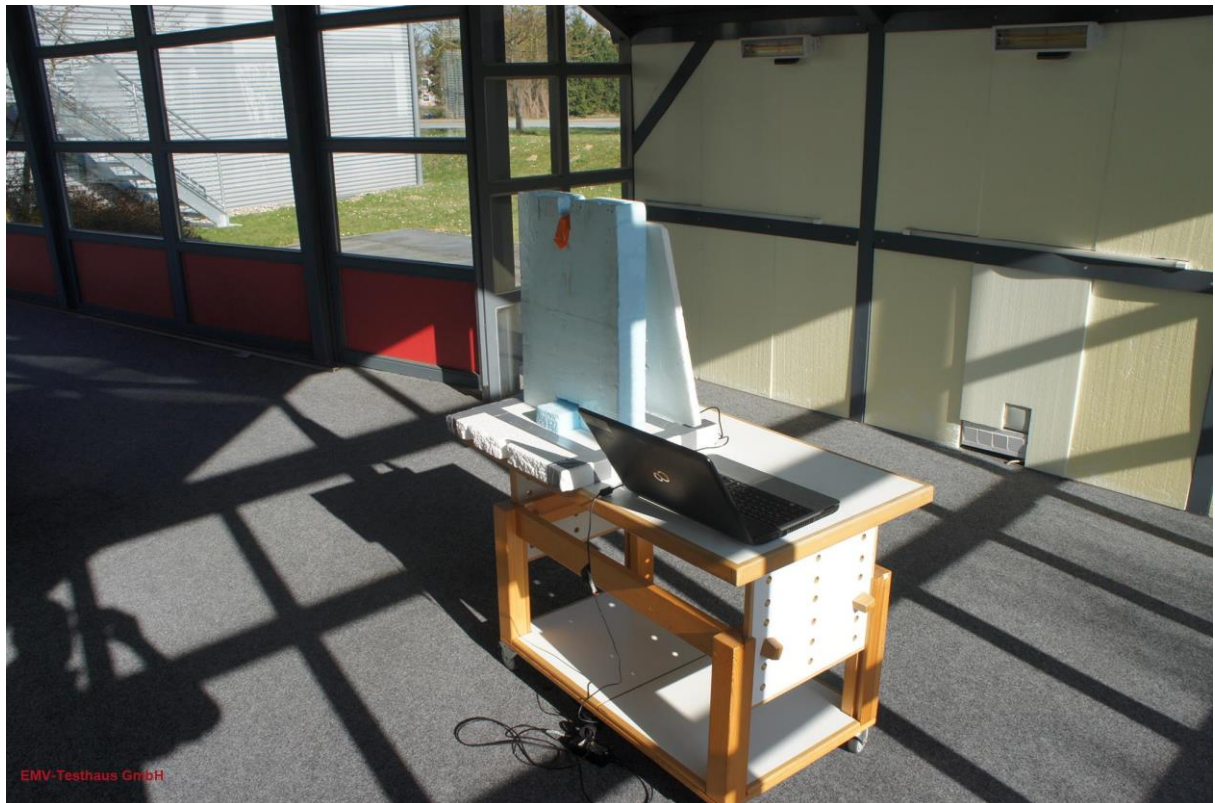
Picture 7: OATS, test setup final radiated emission test (rear view)
