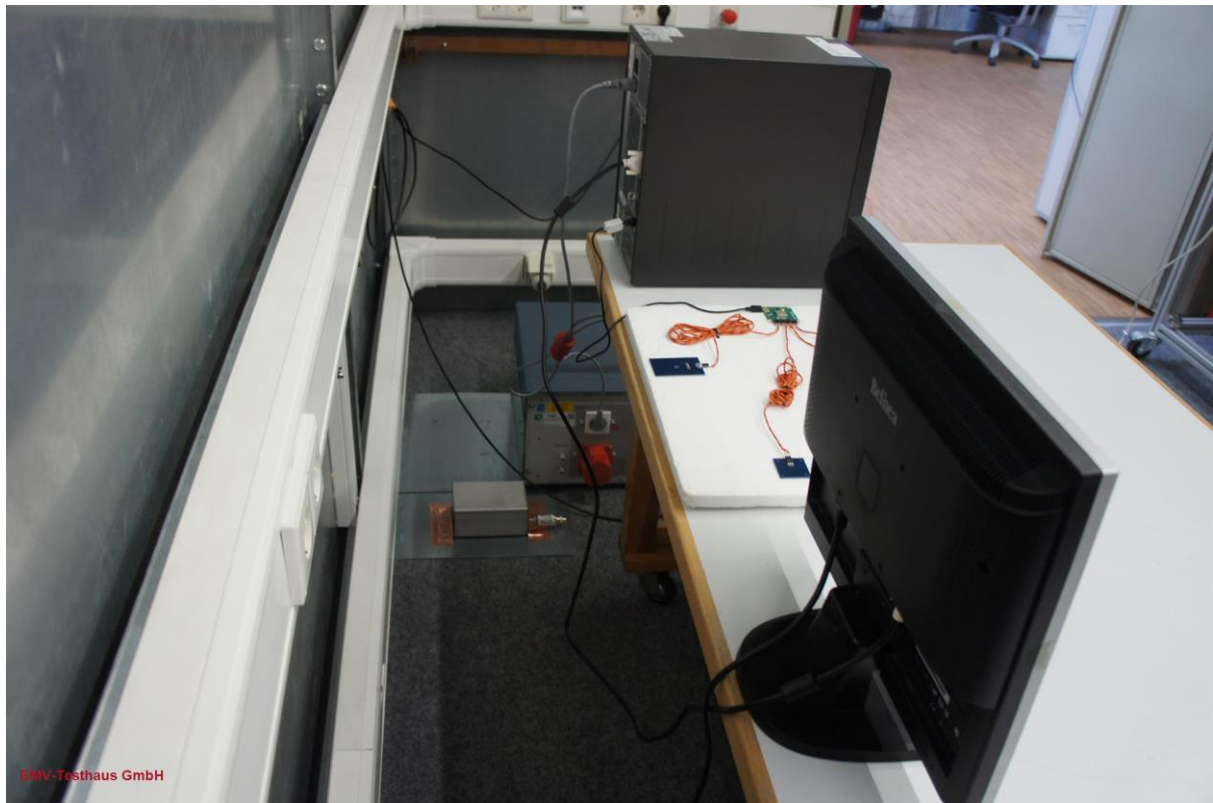
Picture 2: Test setup AC power line conducted emission (rear view)
