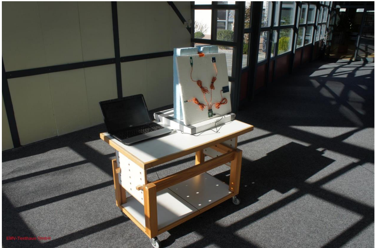
Picture 6: OATS, test setup final radiated emission test (front view)
