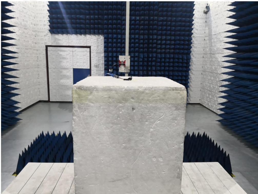
RADIATED EMISSION TEST SETUP ABOVE 1GHZ
