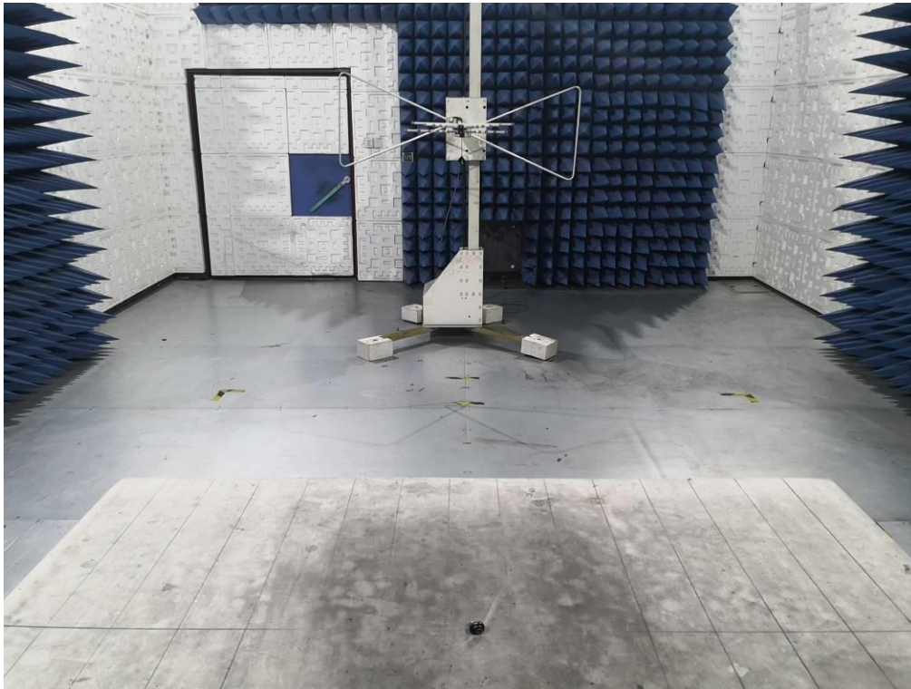
RADIATED EMISSION TEST SETUP ABOVE 1GHZ
