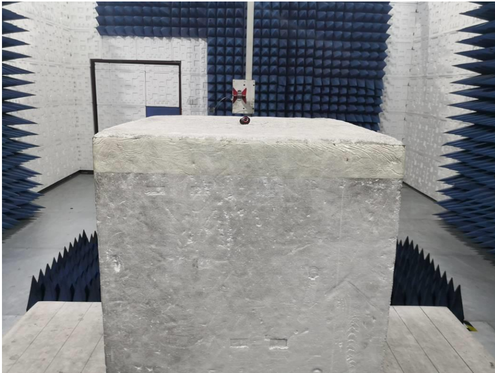
RADIATED EMISSION TEST SETUP ABOVE 1GHZ
