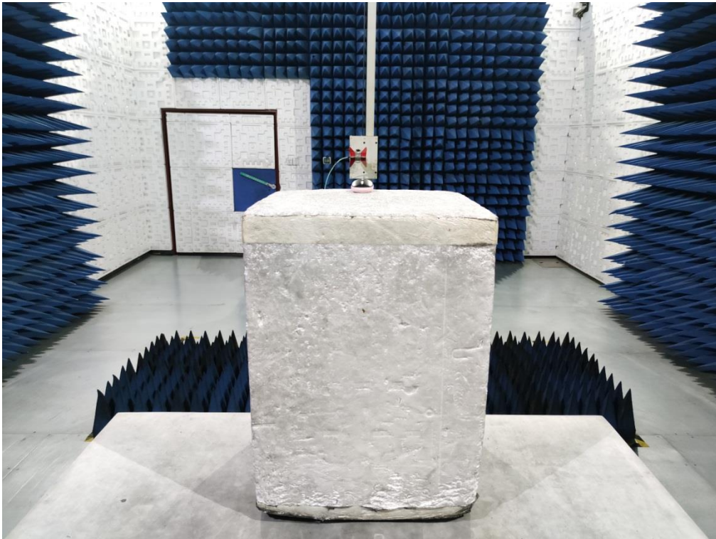
RADIATED EMISSION TEST SETUP ABOVE 1GHZ
