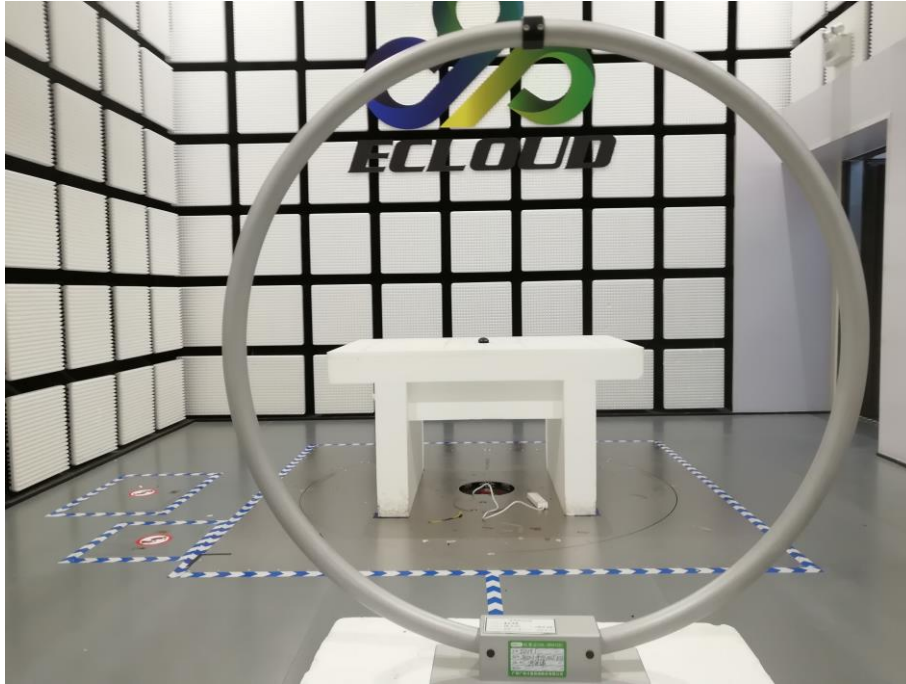
Fig. 1 Radiated emission setup photo(Below 30MHz)
