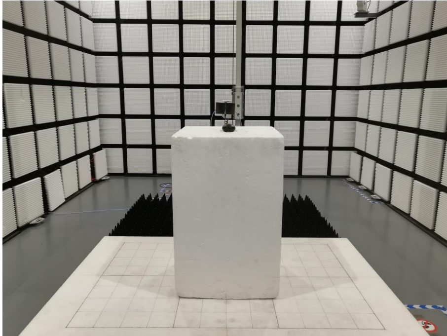
Fig. 3 Radiated emission setup photo(Above 1GHz)
