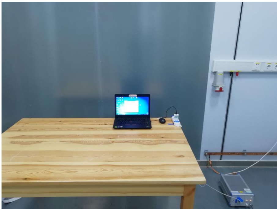
Fig. 4 Power line conducted emission setup photo
