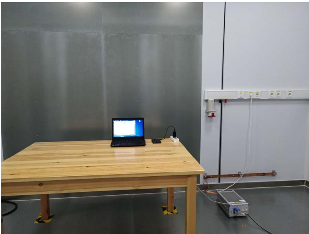
Fig. 4 Power line conducted emission setup photo
