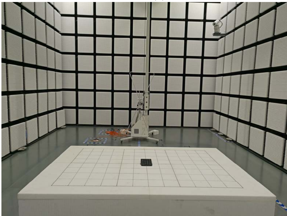
Fig. 2 Radiated emission setup photo(30MHz- 1GHz)
