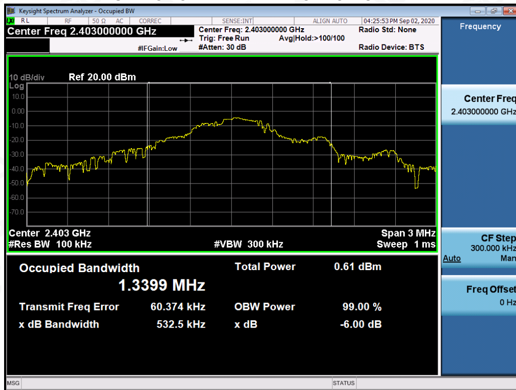
TEST PLOT OF BANDWIDTH FOR LOW CHANNEL
