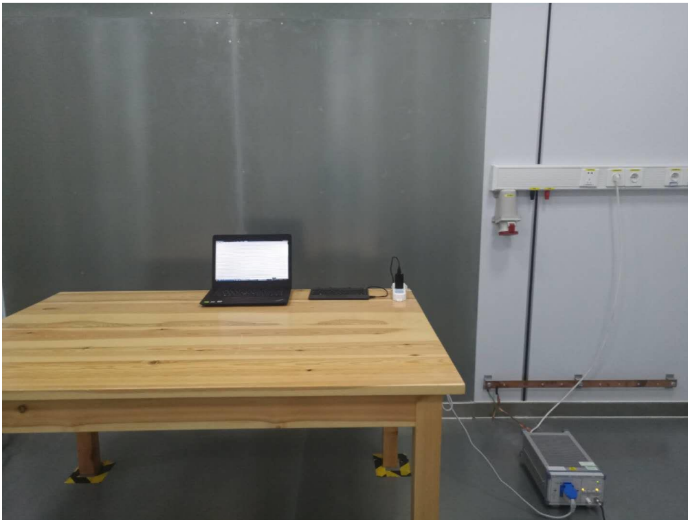
Fig. 4 Power line conducted emission setup photo
