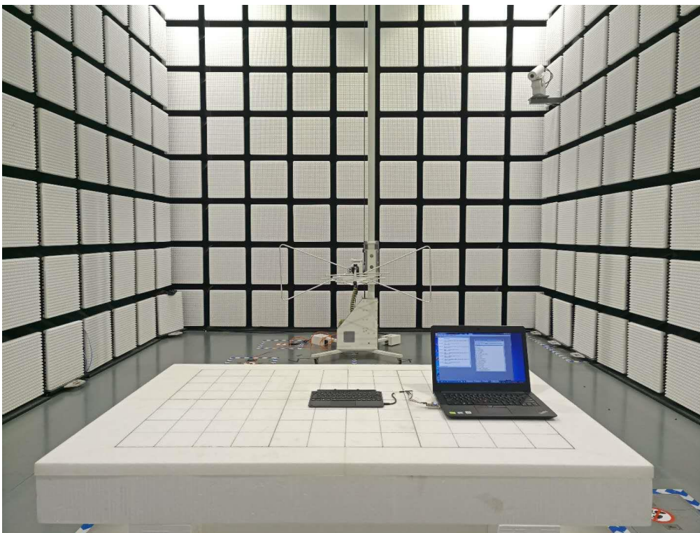
Fig. 2 Radiated emission setup photo(30MHz-1GHz)
