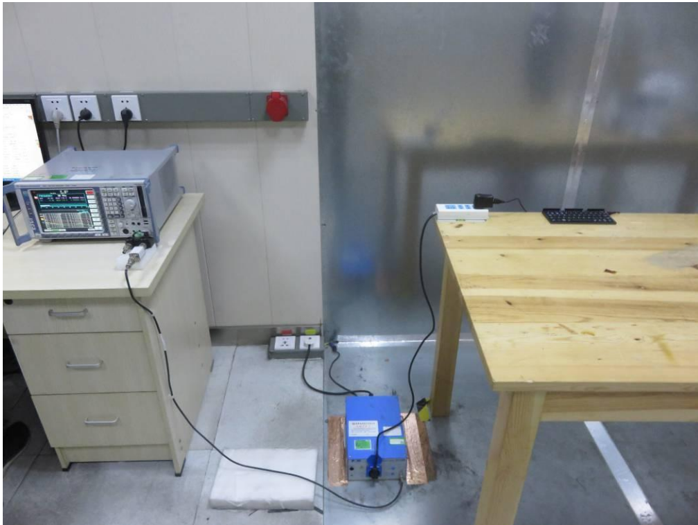
FCC RADIATED EMISSION TEST SETUP
