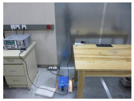
FCC RADIATED EMISSION TEST SETUP
