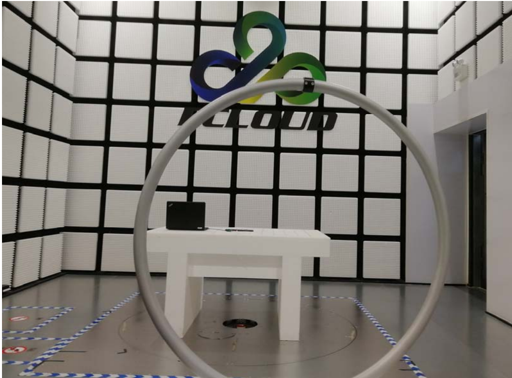
Fig. 1 Radiated emission setup photo(Below 30MHz)
