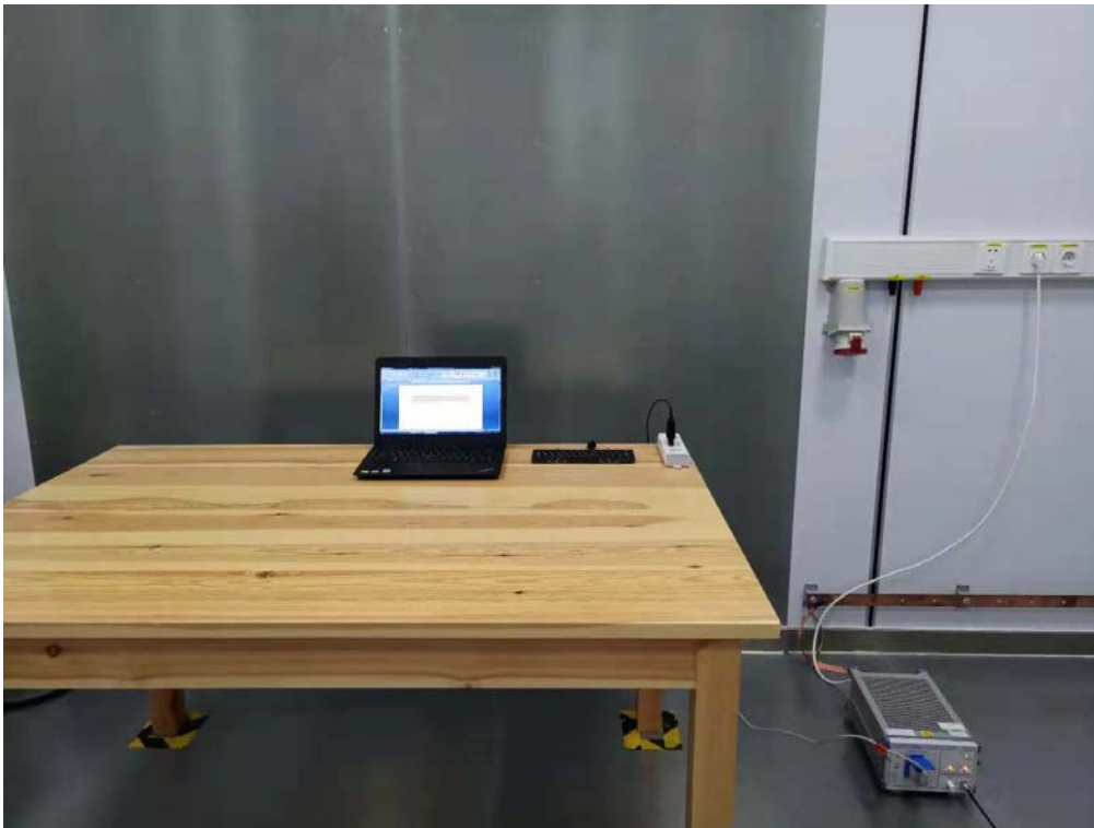
Fig. 4 Power line conducted emission setup photo
