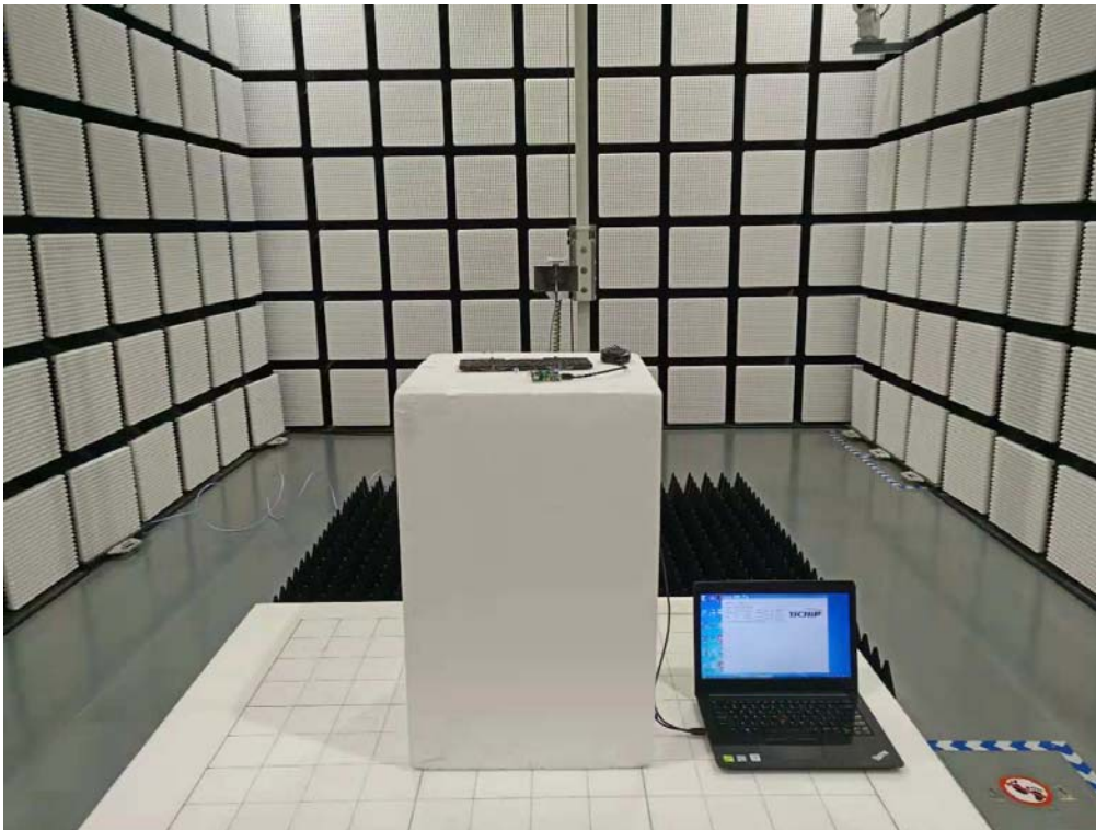
Fig. 3 Radiated emission setup photo(Above 1GHz)
