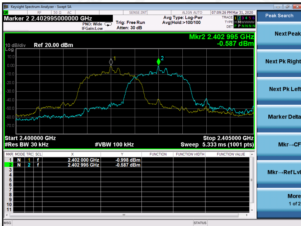
TEST PLOT FOR FREQUENCY SEPARATION
