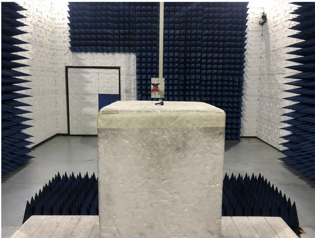
RADIATED EMISSION TEST SETUP ABOVE 1GHZ
