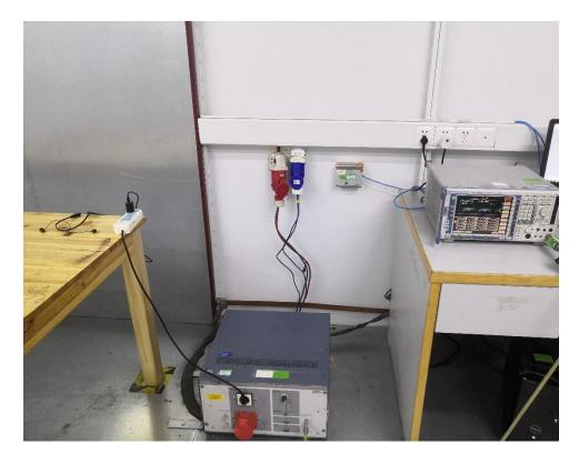
**CONDUCTED TEST SETUP**
