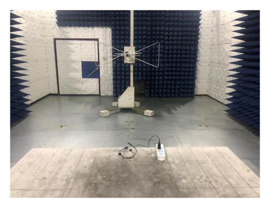
RADIATED EMISSION TEST SETUP ABOVE 1GHZ
