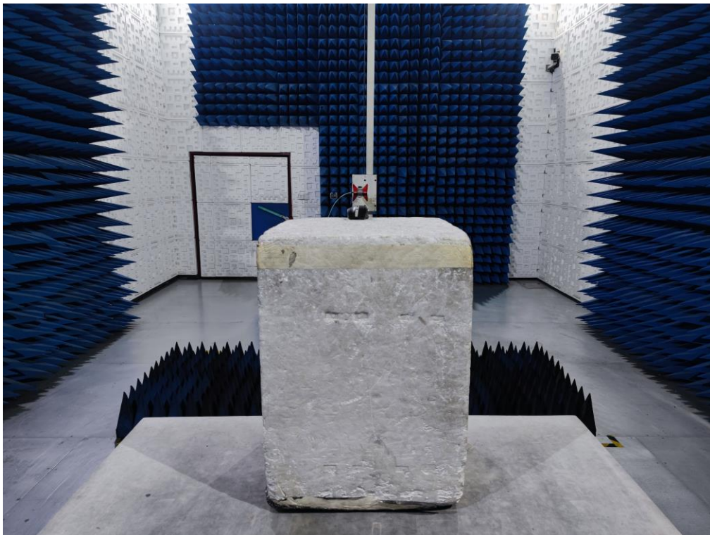
RADIATED EMISSION TEST SETUP ABOVE 1GHZ
