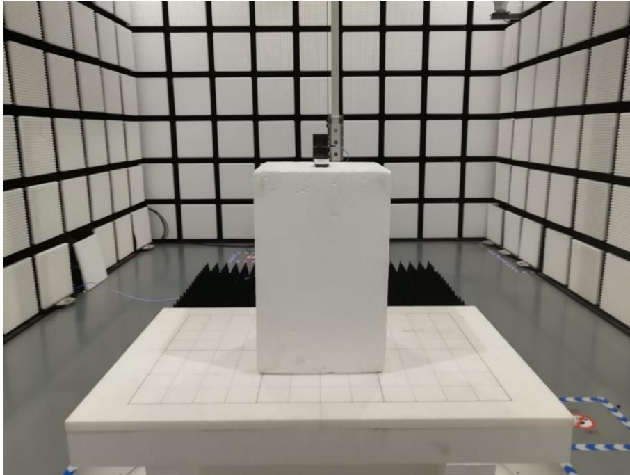
Fig. 3 Radiated emission setup photo(Above 1GHz)
