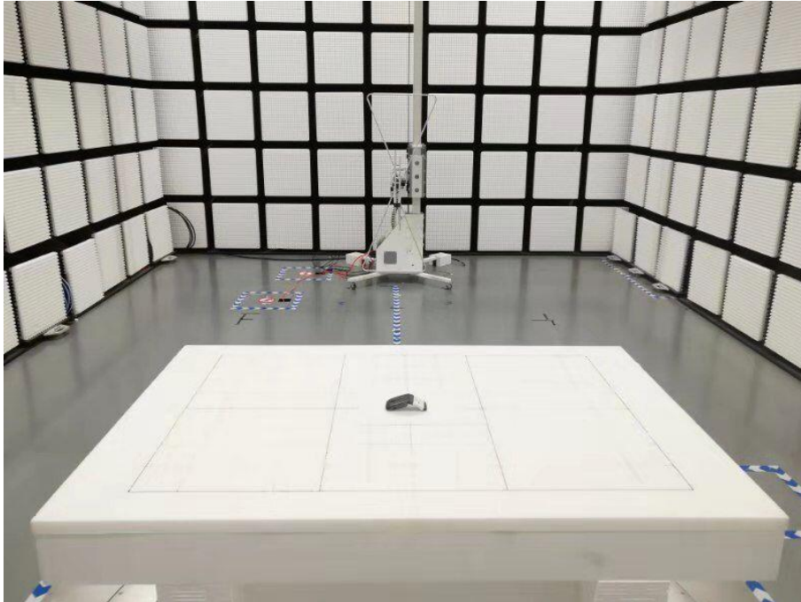
Fig. 2 Radiated emission setup photo(30MHz- 1GHz)
