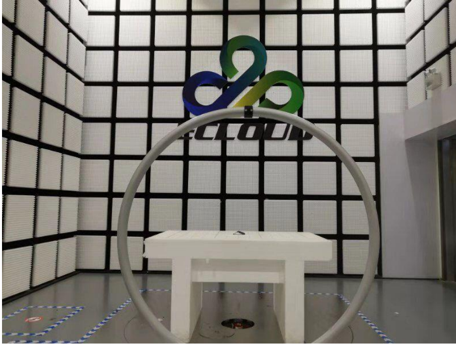
Fig. 1 Radiated emission setup photo(Below 30MHz)
