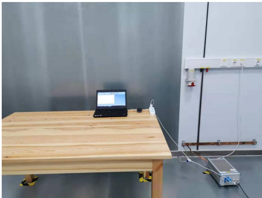
Fig. 4 Power line conducted emission setup photo
