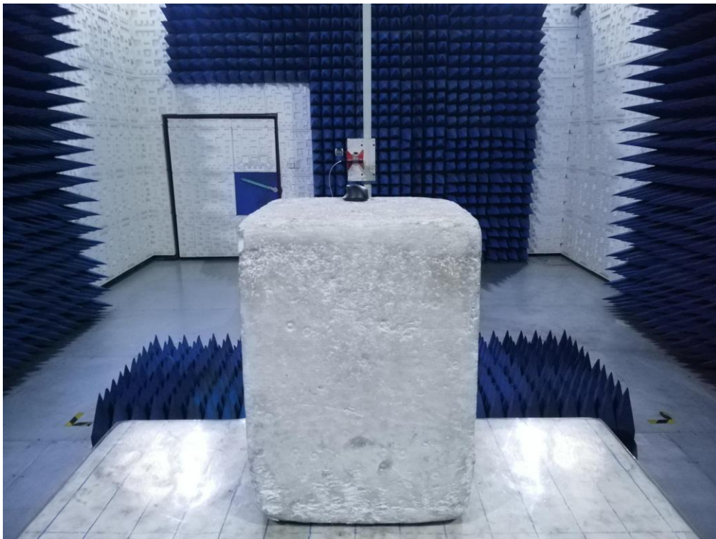
RADIATED EMISSION TEST SETUP ABOVE 1GHz
