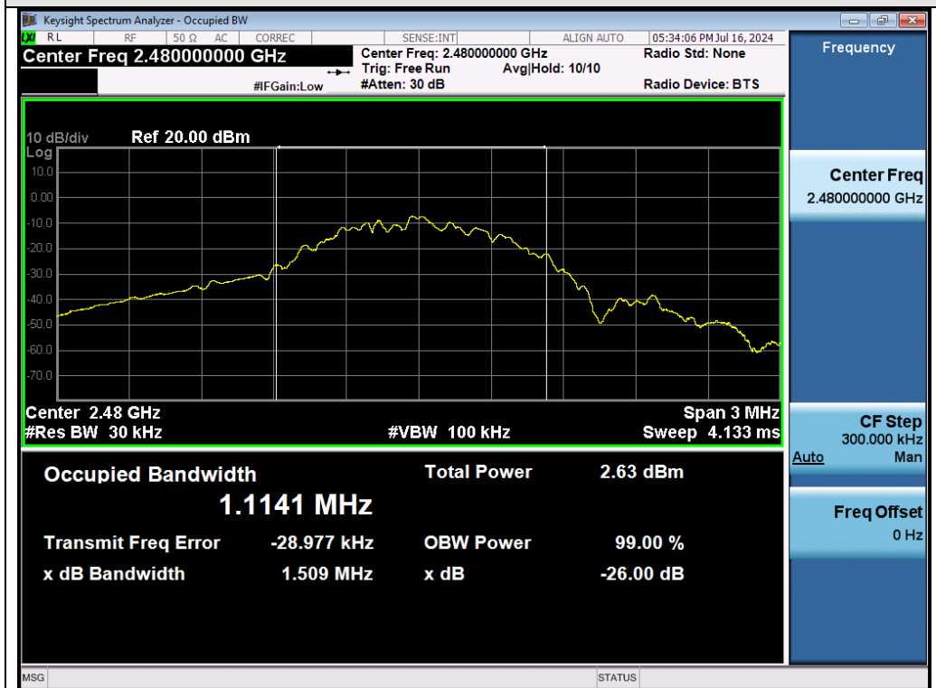
Test_Graph_LE1M_ANT1_2480_1Mbps_OBW
