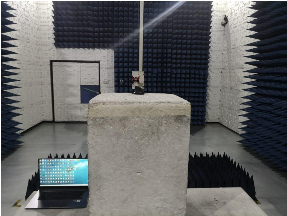
RADIATED EMISSION TEST SETUP ABOVE 1GHz
