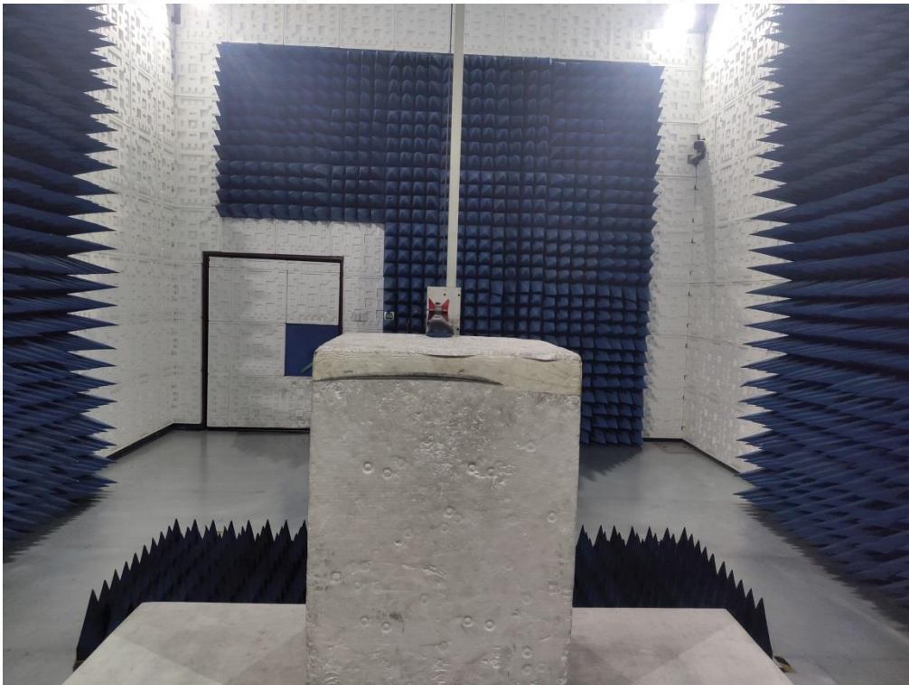
RADIATED EMISSION TEST SETUP ABOVE 1GHZ
