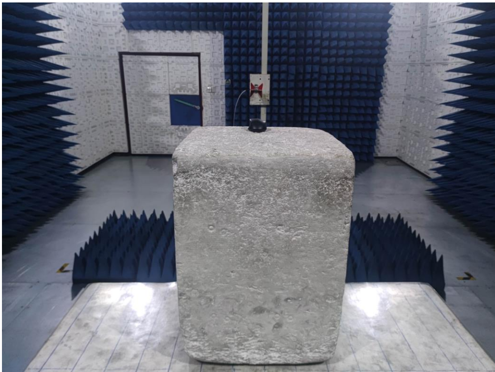
RADIATED EMISSION TEST SETUP ABOVE 1GHz
