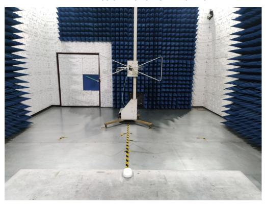
RADIATED EMISSION TEST SETUP ABOVE 1GHz
