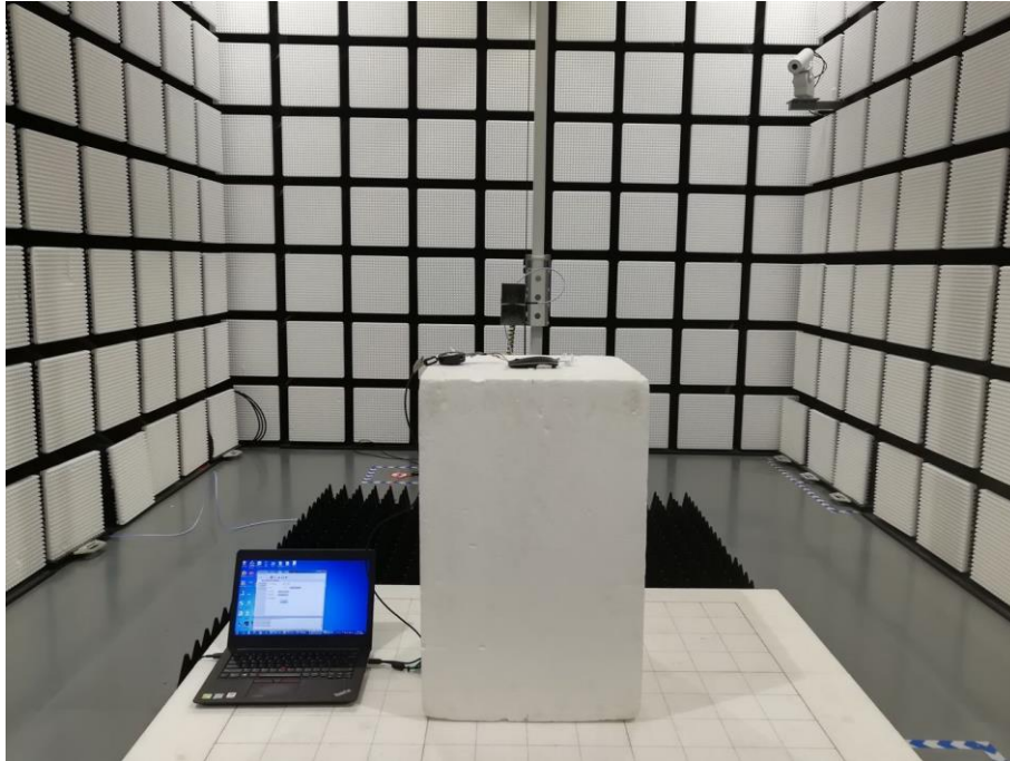
Fig. 3 Radiated emission setup photo(Above 1GHz)
