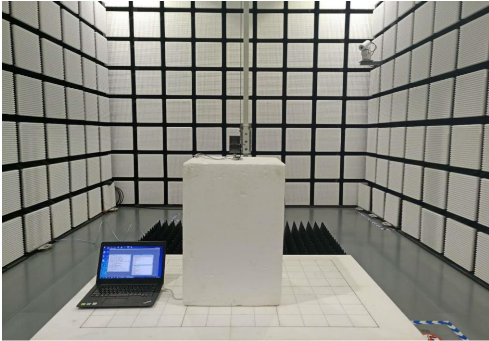
Fig. 3 Radiated emission setup photo(Above 1GHz)
