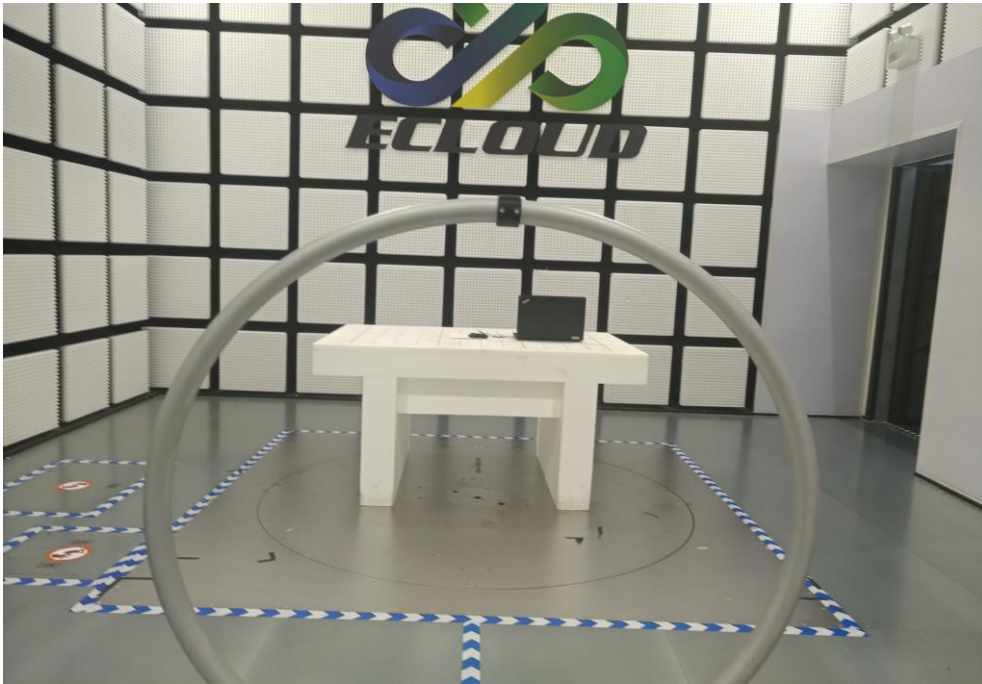
Fig. 1 Radiated emission setup photo(Below 30MHz)
