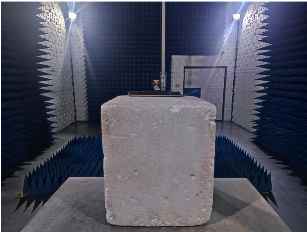
RADIATED EMISSION TEST SETUP ABOVE 1GHz
