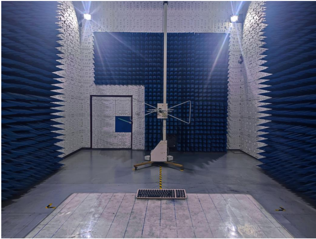
RADIATED EMISSION TEST SETUP ABOVE 1GHz
