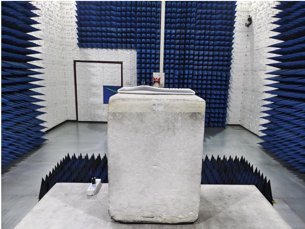
RADIATED EMISSION TEST SETUP ABOVE 1GHz
