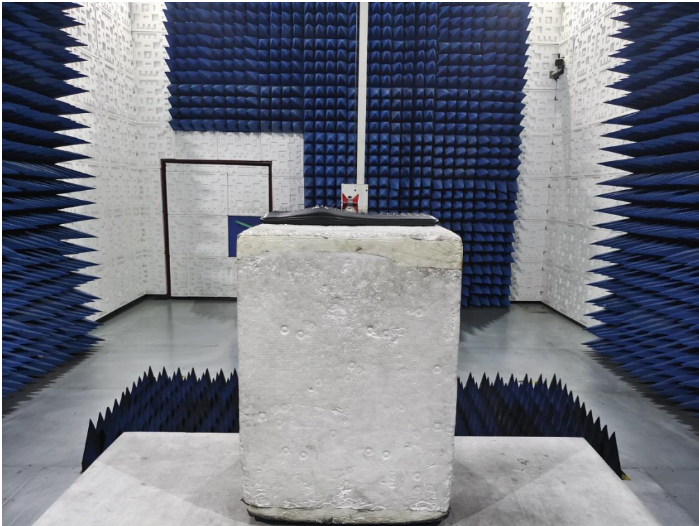
RADIATED EMISSION TEST SETUP ABOVE 1GHZ
