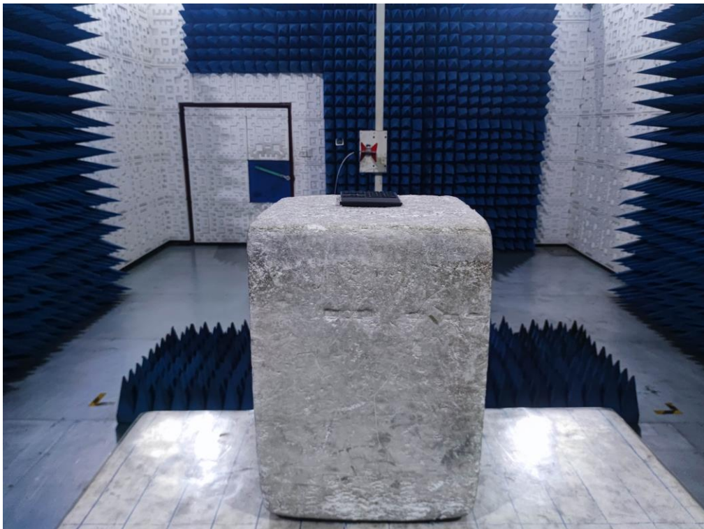
RADIATED EMISSION TEST SETUP ABOVE 1GHz
