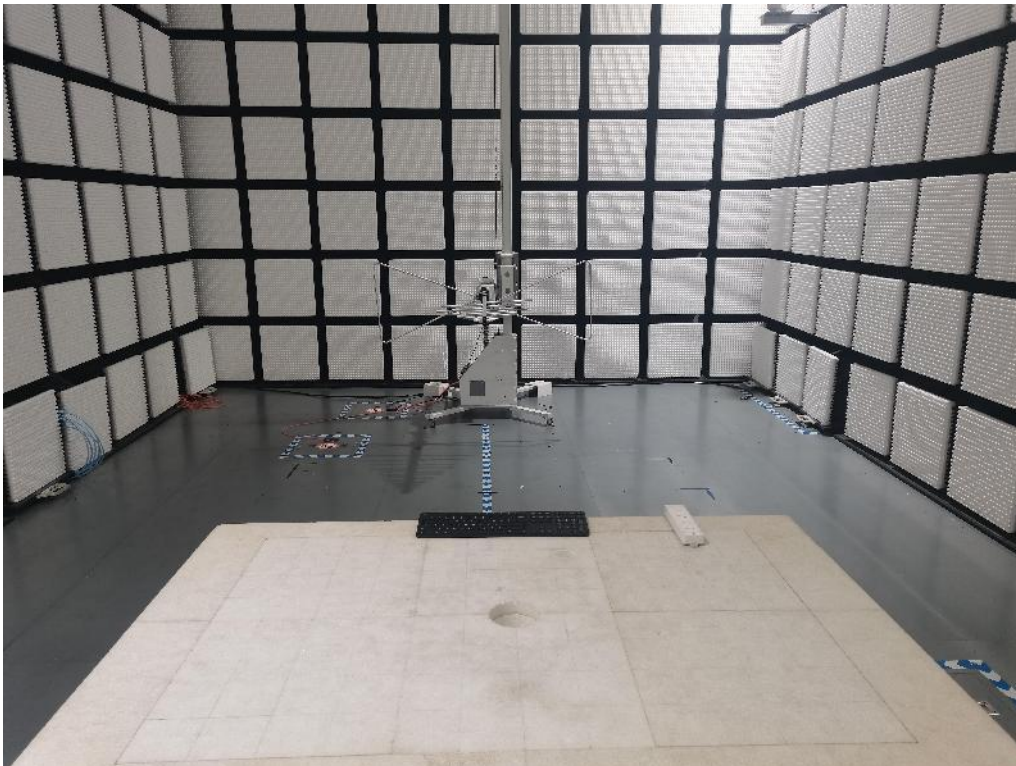
Fig. 2 Radiated emission setup photo(30MHz- 1GHz)
