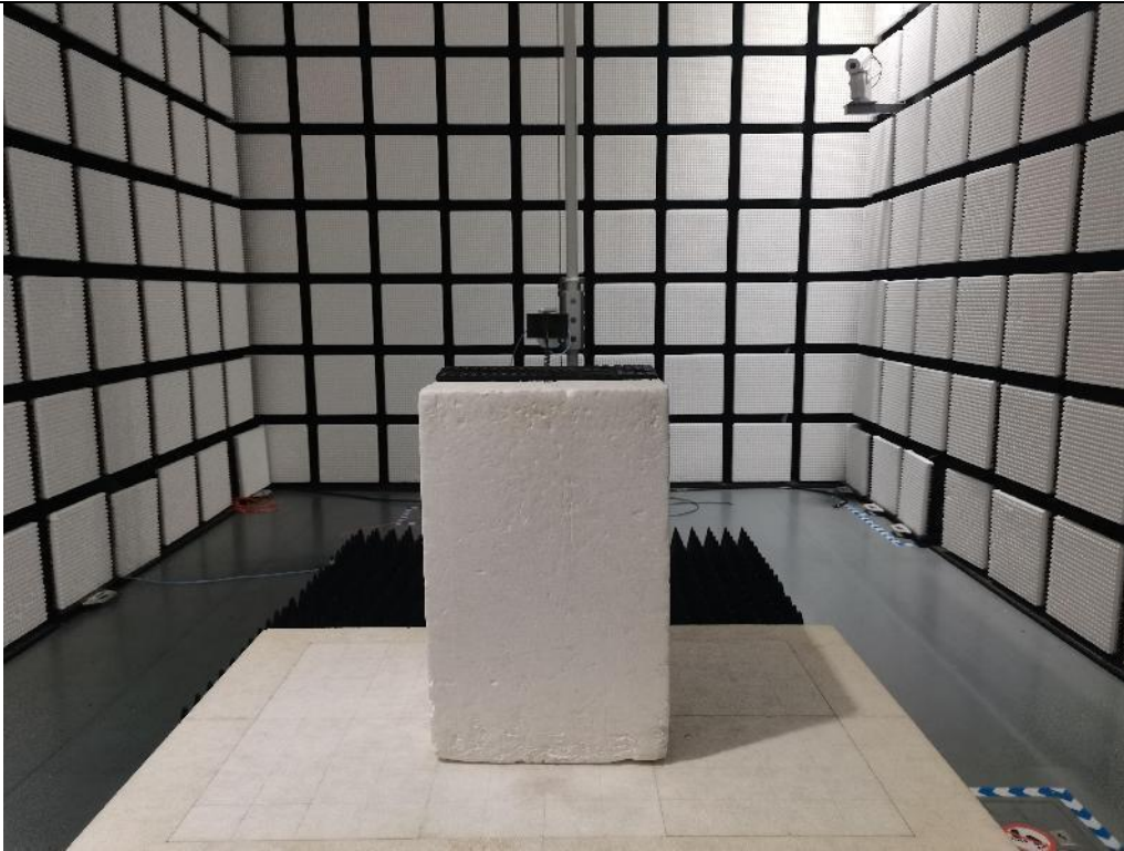
Fig. 3 Radiated emission setup photo(Above 1GHz)
