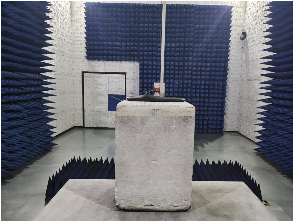
FCC RADIATED EMISSION TEST SETUP ABOVE 1GHZ
