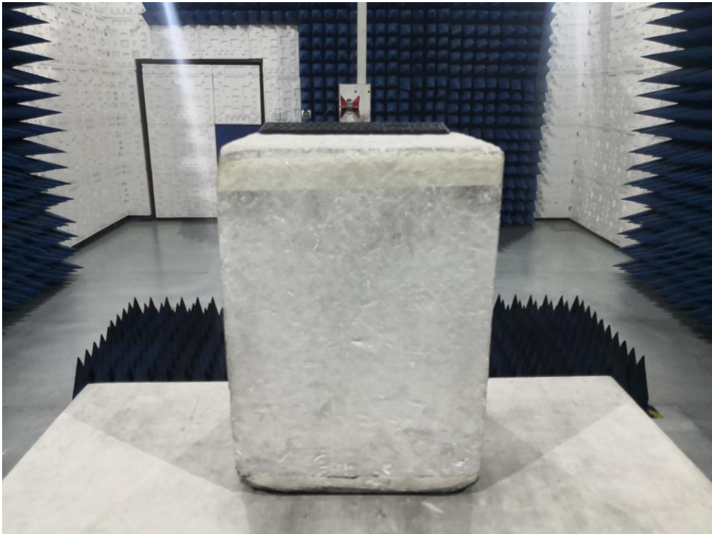
RADIATED EMISSION TEST SETUP ABOVE 1GHZ
