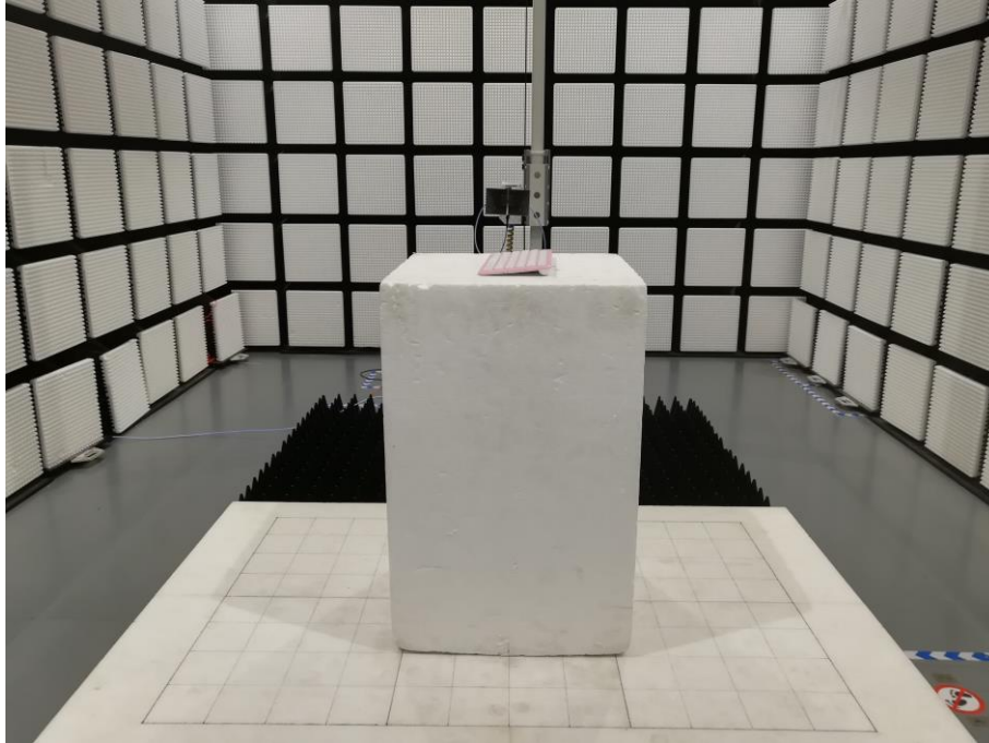
Fig. 3 Radiated emission setup photo(Above 1GHz)
