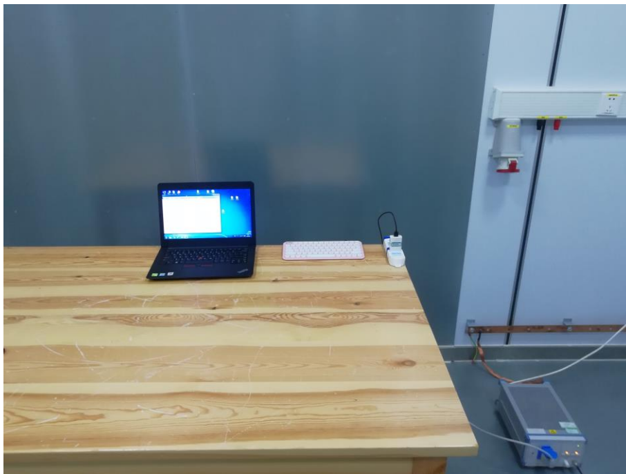
Fig. 4 Power line conducted emission setup photo
