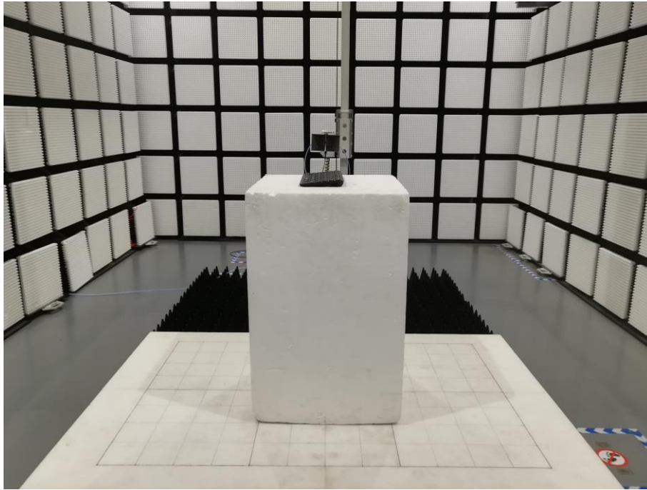
Fig. 3 Radiated emission setup photo(Above 1GHz)
