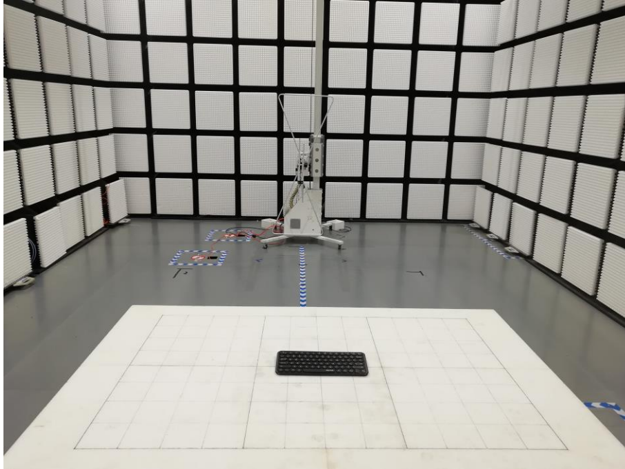
Fig. 2 Radiated emission setup photo(30MHz- 1GHz)
